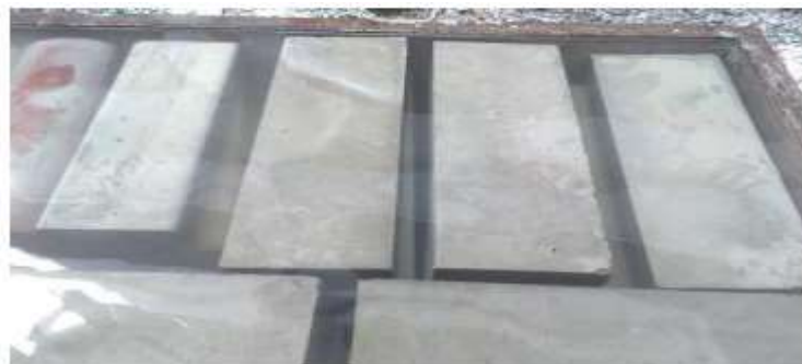
Figure 5 Curing of RC beams
